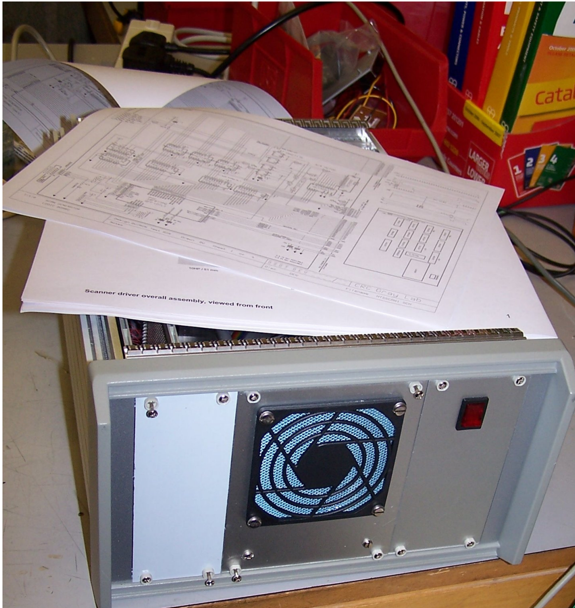
Figure 13. The scanner driver during construction. Yes, we did use the same circuits as shown earlier!
