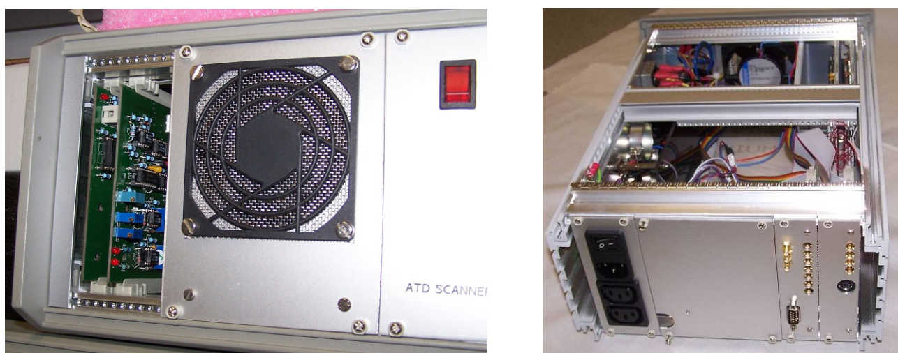
Figure 1. The scanner driver unit, from the front (left), with a panel removed to show the circuit boards and the rear. Interface signals are on the right of the right hand image and AC power connections are on the left. We provide two further IEC mains outputs for ancillary equipment as there are never enough mains sockets, even in the best laid out laboratory!
